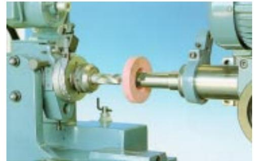
MILLING CUTTER END GRINDING
