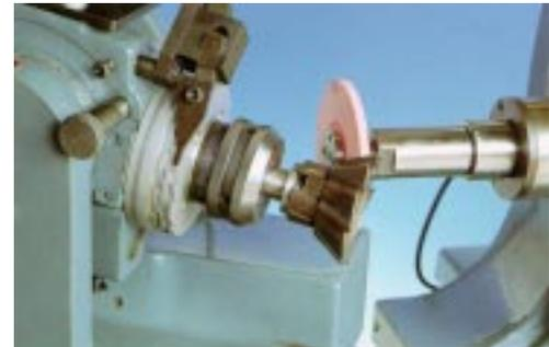
FORMED MILLING CUTTER GRINDING
