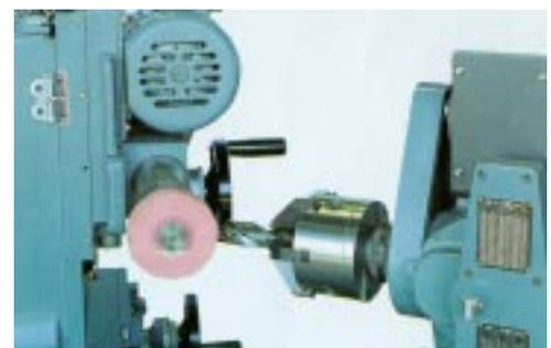
DRILL BIT GRINDING
